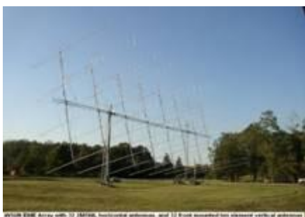
Which EME Array with 12 J4100, horizontal antennas, and 12 EME horizontal for element vertical antennas
