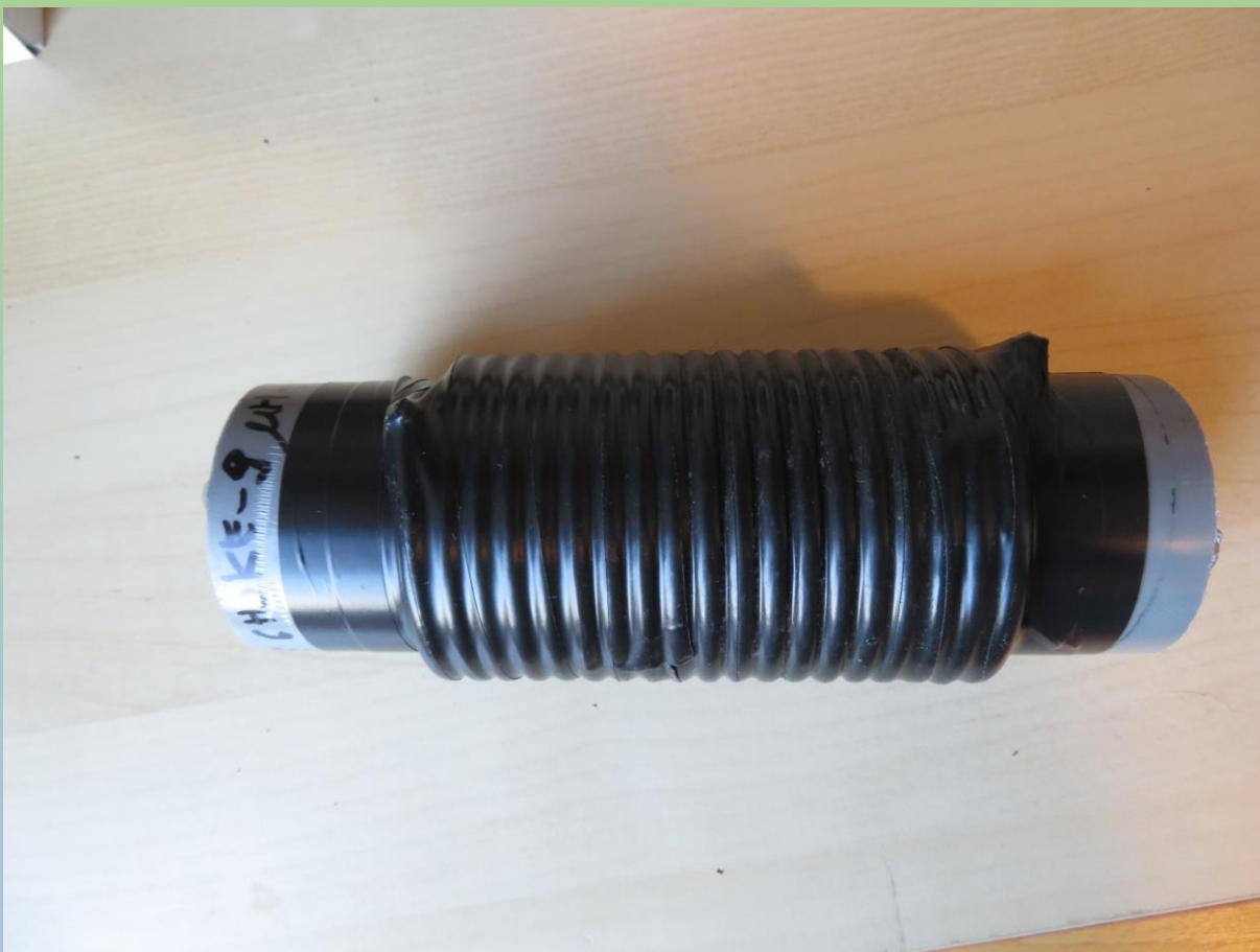
RF choke: 19 w RG-58 op PVC diameter 5 cm
